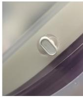
3. Ensure the DLC Front alignment hole is centered on the Front Turn Clip.
