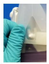
5. Pull each DLC side down towards the Helmet back and tightly against the white foam strip, position each side DLC Mounting Hole as centered as possible over each respective FCC side Mounting Post.
