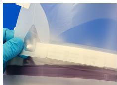
4. The DLC Front Alignment Hole secured, grasp one DLC end by the Flapper and stretch it tauntly until that side Mounting Hole is over that side Mounting Post.
