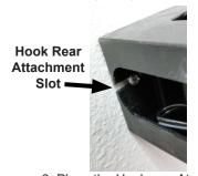
3. Place the Hook rear Attachment Slot over the bottom screw already in the wall anchor. For a snug fit of the Hook to the wall, if the screw is too close to the wall, loosen it. if the screw is too loose, tighten it.
