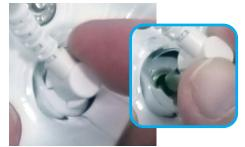
1. Ensure the Power Cord Connector notch is aligned with the Helmet Cord Connector indent, grasp the Cord Connector out and away from the Helmet.
