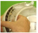
3. With thumb against bottom front of Helmer, pull fingers down and push thumb up to disengage Front Snaps.
