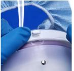
3. Align FCC front TurnClip horizontally, lift the DLC2 Lens Front Alignment Hole off the TurnClip.
