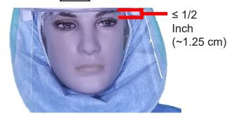
**Condition 1:** Position the Helmet so that the front headband is within ½ inch of the eyebrows and the rear headband is resting under the occipital bone above the vertebrae on the neck, and then tighten the Adjustment Knob clockwise to ensure the most secure fit of the helmet on the head for all activities. Do not over tighten to cause discomfort.
