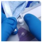
2. Align and snap one DLC2 Side Attachment Hole over the respective FCC Side Attachment Post. Repeat for other side.
