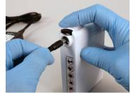
3. Connect a powered on Battery Charger connector to the Battery. Push connector into Battery receptacle fully - Do NOT push down on the Battery Secure Lock (Black) button.
