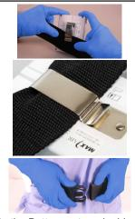
Belt. Place top edge of Belt under the Battery Clip, up to the Clip top, so the Clip Detent rests on the Clip Base and NOT the Belt. Place the belt comfortably around the waist with the battery near the side-back of the right hip.
