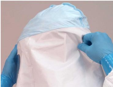
11. Continuing process of 10, pull Hood all the way down so that Hood Filter (blue) is fully down on Helmet.
