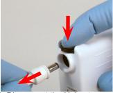
Disconnect the Helmet Power Cord from the Battery - Press down on the Secure Lock (Black) Button to release, then pull the cord connector out from the Battery connection receptacle.
