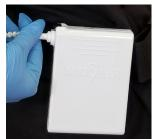
9. Connect Helmet Power Cord to Battery. Push Power Cord Connector into Battery Receptacle until Secure Connection audibly clicks.
