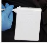
Cord to Battery. Push Power Cord Connector into Battery Receptacle until Secure Connection audibly clicks.
