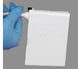
7. Connect the Helmet Power Cord to the Battery by pushing its Connector into the Battery Receptacle until the Secure Connection audibly clicks.
