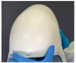
Align the front centerline of the HFR FCC with the front centerline of the Hood and position the HFR FCC over the Hood so that both front bottoms align.
