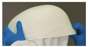
Hold the underneath back of the Helmet steady with the thumb while pulling the back of the HFR FCC fully down to even with the bottom rear of the Helmet.
